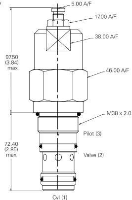
Note: For applications above 210 bar - please consult our technical department or use the steel body option. Note: Tightening torque of "F" adjuster locknut - 20 to 25 Nm.
