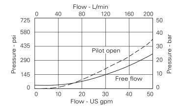
Note: This valve has been designed to eliminate instability from flexible boom applications or where the load induced pressure varies greatly. To get the best results, the settings should be adjusted for each application and then factory set for production quantities. Please contact Eaton/Integrated Hydraulics for more information.
