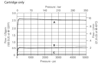
A - 9,5 L/min (2.5 USgpm) B - 1,9 L/min (0.5 USgpm)
