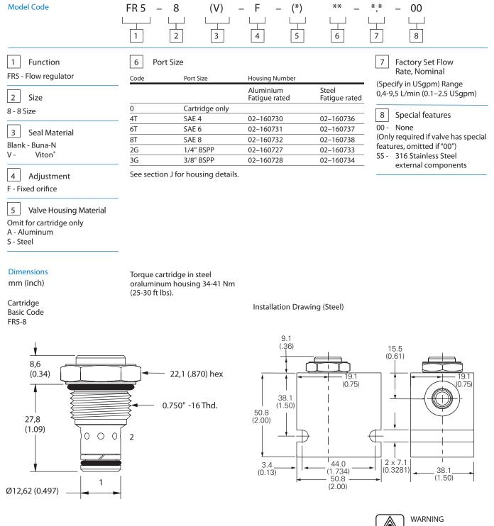
Aluminum housings can be used for pressures up to 210 bar (3000 psi). Steel housings must be used for operating pressures above 210 bar (3000 psi).
