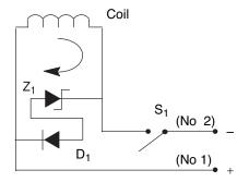
NOTE: These surge suppression devices are "Polarity Dependent." Proper biasing conditions must be met when installing/connecting a coil in a system.
