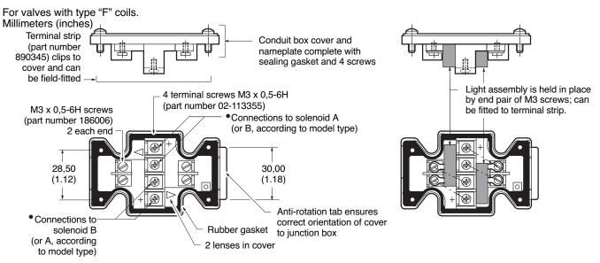
For DC coils the +ve lead(s) must be connected to the terminal(s) marked +. When using 3-wire incoming leads to double solenoid valves (i.e. common neutral) the inner pair of terminals must be interconnected  For correct light indication of energized solenoid ensure that solenoid leads are correctly connected: light terminals are common with each outer pair of solenoid terminals according to the side with + mark.
