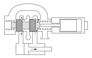
Pressure surges can occur within the armature tube of 2-land wet armature valves due to cylinder port decompression. These surges can easily exceed tube pressure rating and result in premature tube failure.
