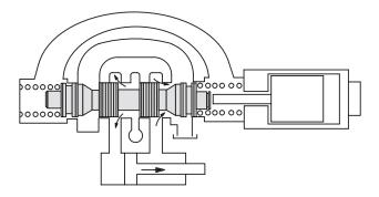
The armature tube area is isolated from the tank port area by the outboard lands on the 4-land spool. Tank port pressure surges do not reach the armature tube to cause failure.
