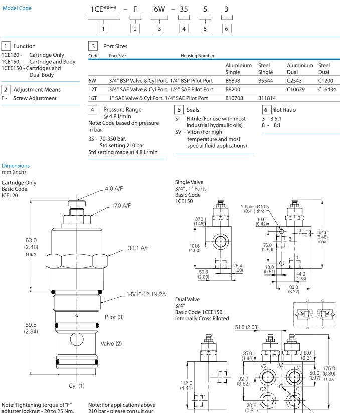
adjuster locknut - 20 to 25 Nm.
